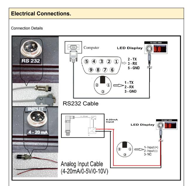
Connect the 4-20ma current loop /0-5v DC/0-10v DC to the analog input cable.
